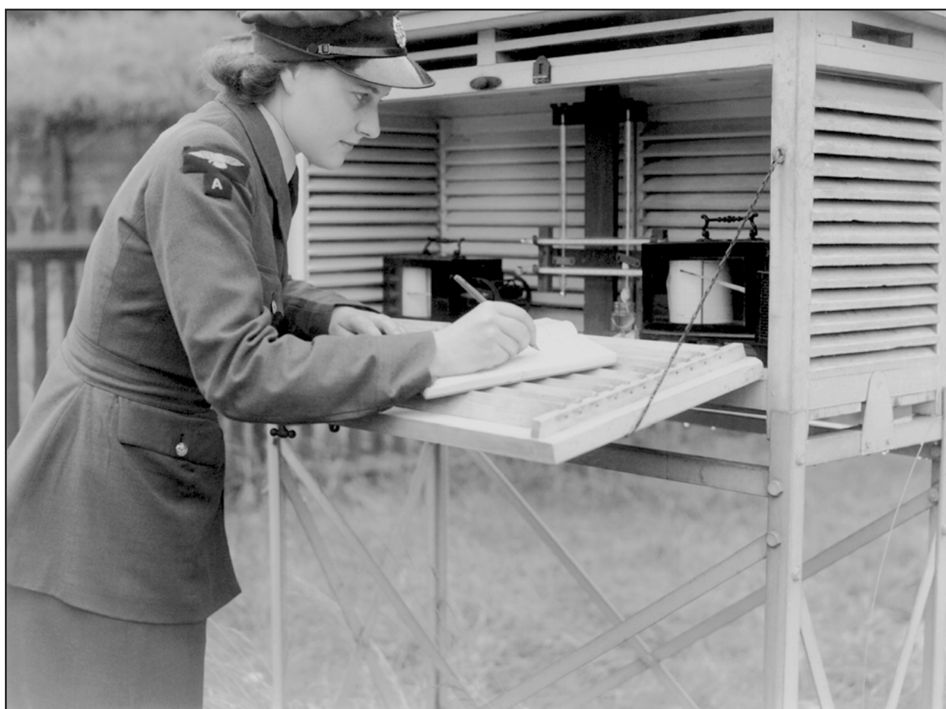
Figure 15. A Met WAAF reads wet and dry thermometers housed in a Stevenson Screen – some of the thousands of instruments produced at Stonehouse.
