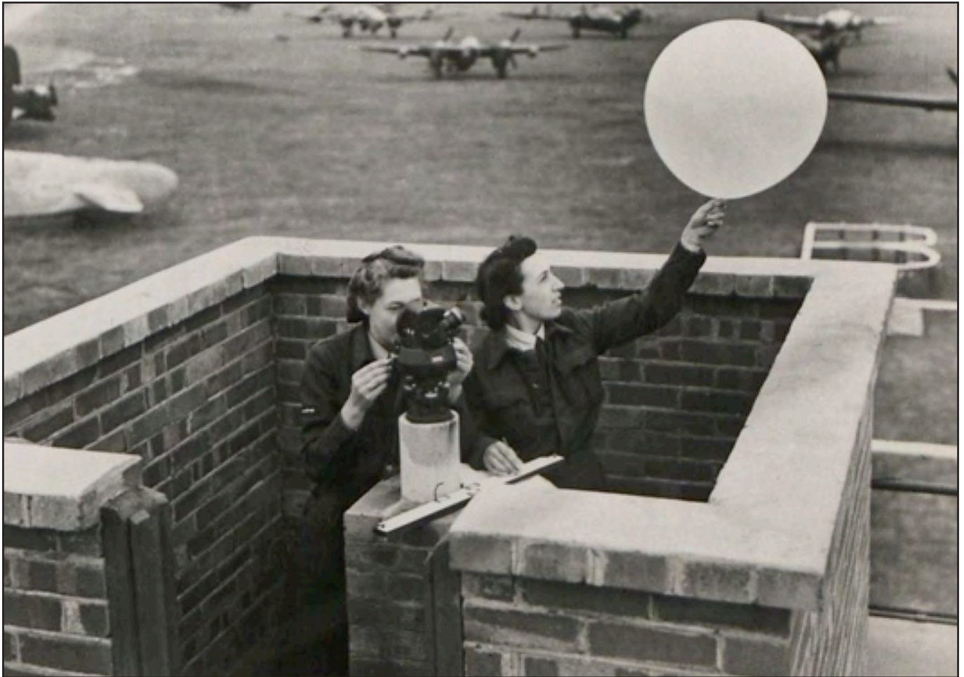
Figure 16. Two WAAF personnel taking upper air observations with a balloon, theodolite and slide rule.
