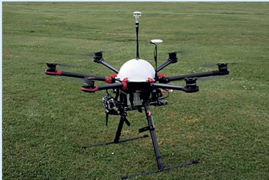
An instrumented Unmanned Aerial Vehicle (UAV) developed at the Met Office boundary-layer research facility in Cardington, UK. The UAV is equipped with instrumentation to make high-resolution vertical profile measurements of temperature, humidity and wind through the depth of the boundary layer.
