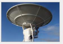
A device that sends out electromagnetic pulses which detect objects in the sky, like raindrops, and can tell how big they are, where they are and how fast they are falling.
